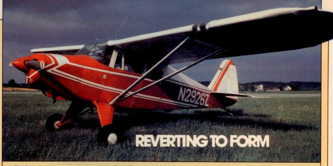
The Piper Pacer is a source of hours of enjoyment for trivia hunters and students of the marque. The first Pacer, the PA-20, was a mildly changed Clipper. It started with a Lycoming O-235 engine, rated at 108 hp; the Pacer 115 had no flaps (as the end-of-the-tube-and-fabric Pipers, the Colt, was configured) and had a gross weight of 1,750 pounds. (See "Short-Wing Pipers", November 1981 *Pilot*, p. 117.)
