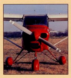
The 150-hp Lycoming O-320-A1A increased the airplane's cruise speed only a couple of knots but improved its rate of climb by approximately 100 fpm. Fuel capacity in the Tri-Pacer was increased from 36 gallons to 44 gallons by the addition of an optional auxiliary fuel tank under the rear seat.
